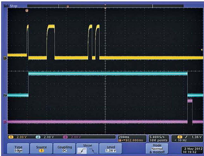
2. The yellow trace (Channel 1) is U1, pin 12, which is configured as an output of PWREN# signal. The blue trace (Channel 2) is the Q output of U2. The purple trace (Channel 3) is the Q output of U3.
