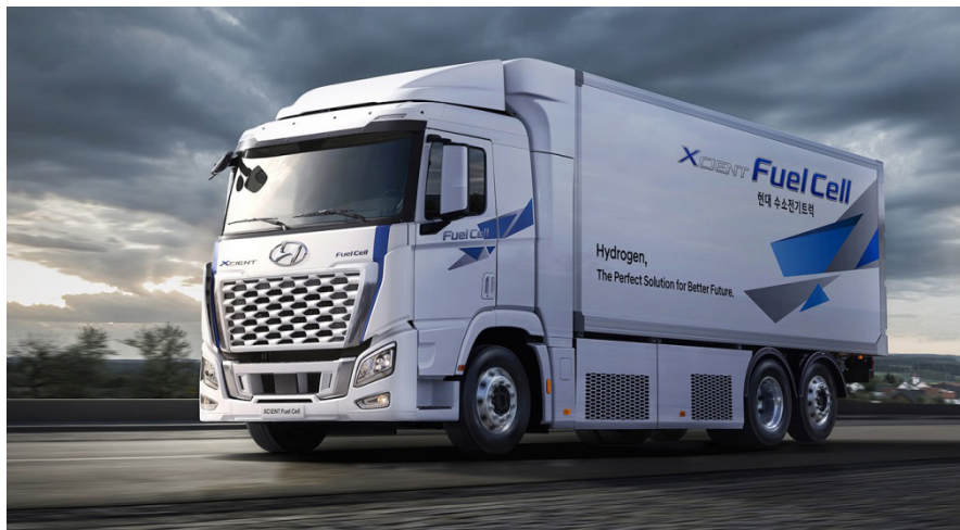
2. The heart of the XCIENT truck is its fuel cell—a twin array of 90-kW stacks—that delivers 180 kW of power and a driving range of 400 km (Source: Hyundai Motor Co.)
