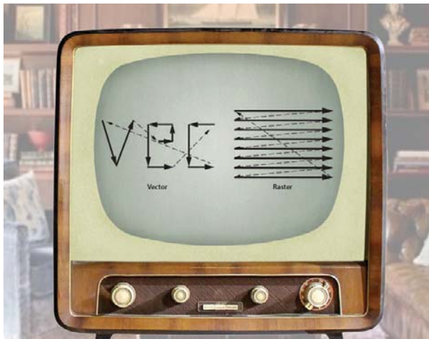
1. A cathode ray tube can display vector and raster images depending on the drive electronics. Credit: Cebas, Dreamstime
