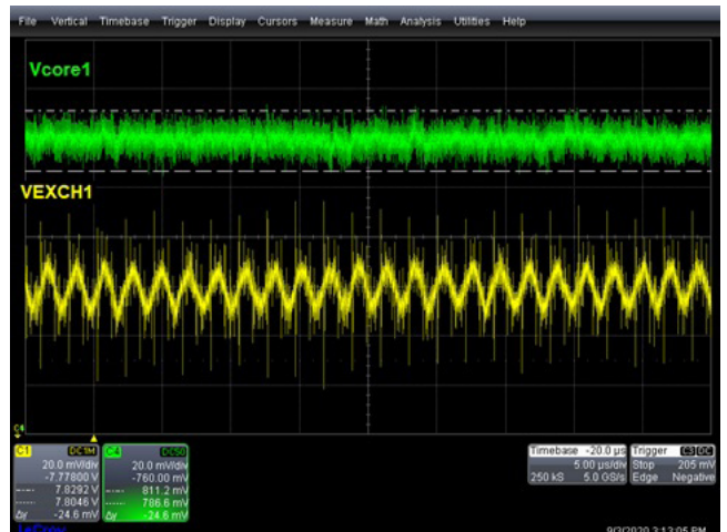
8. Voltage ripple on Vo1 (~25 mV) and floating Vin1 (~70 mV) for the system with the proposed differential Energy Exchanger from Figure 3.
