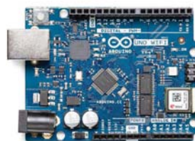
3. The Arduino Uno WiFi uses a module to provide wireless support.
