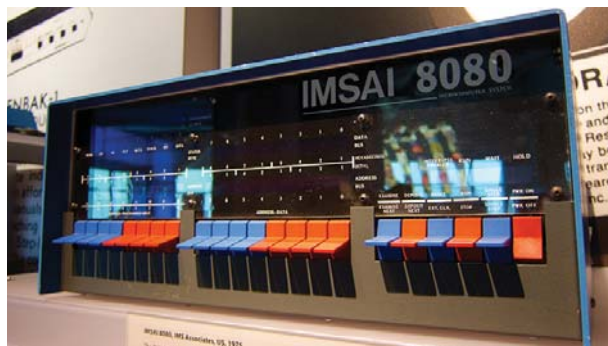
2. The IMSAI 8080 is housed an Intel 8080 microprocessor with S-100 cards providing peripheral and memory support. (Courtesy of Wikipedia, Don DeBold)
