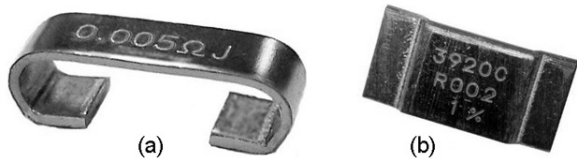
3. Illustrated are an open-air format metal-alloy resistor (a), and a flat-chip format metal-alloy resistor (b).
