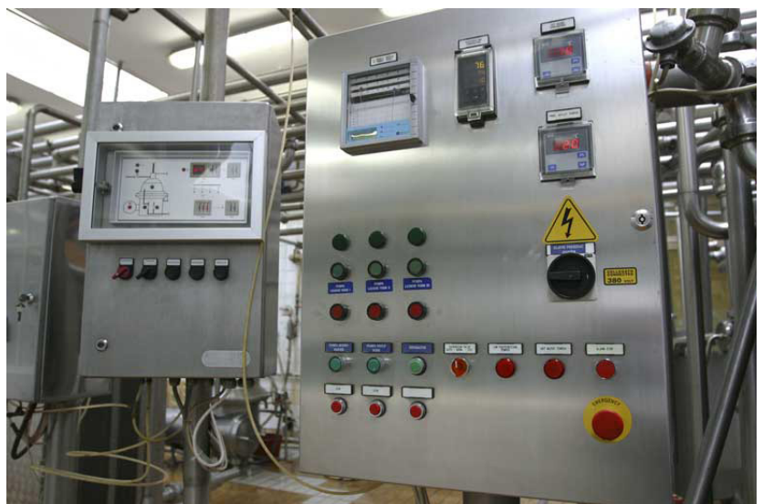
1. Electronic systems intended for use in challenging environments must be able to handle moisture, dirt, vibration, shock, and thermal situations.
