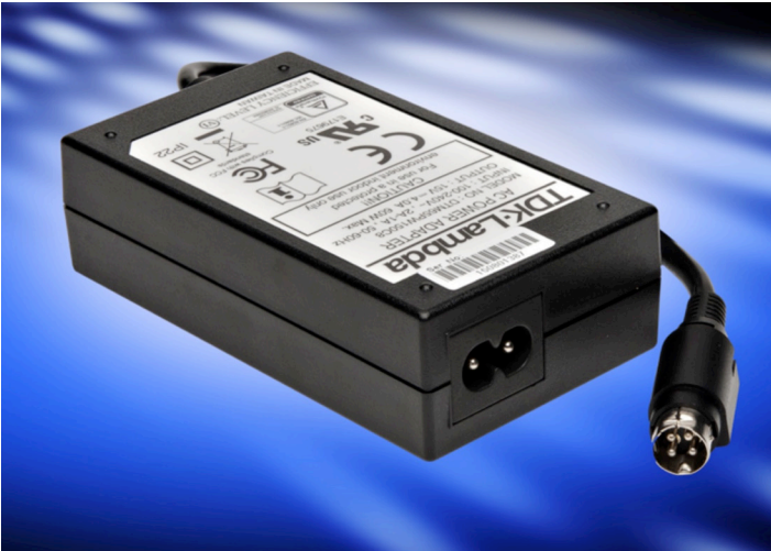
6-4. TDK-Lambda’s medically certified DTM65-C8 external power supplies offer a class II input and do not require an earth ground connection and meets the stringent Level VI DoE standards for efficiency. It is housed in a rugged, vent-free IP21 rated enclosure, measuring 106 x 60 x 31mm. AC is applied using a standard IEC60320-C8 cable and DC provided through a four pin Power-DIN connector.
