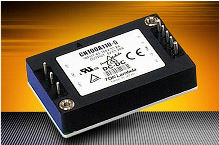
4-1. TDK-Lambda’s CN-A Series of dc-dc converters have a 60V to 160VDC input range with output voltages from 5V to 24VDC (adjustable \pm 10\% ). Output power ratings are 30W, 50W, and 100W. These isolated power modules are in the industry-standard quarter-brick footprint.
