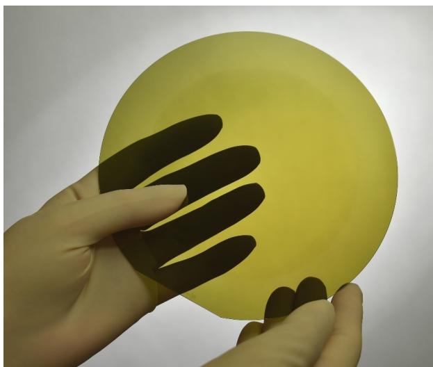
1. Silicon carbide (SiC) is a wide-bandgap semiconductor material with a wider energy difference. Thus, it has higher thermal and electronic properties when compared to traditional silicon. (Source: onsemi)
