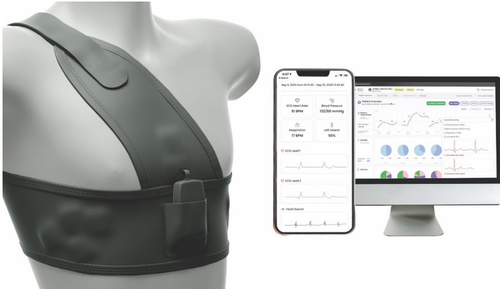
1. Textile-based medical monitor using a smartphone for Bluetooth wireless data. (Courtesy of Nanowear Inc.)
