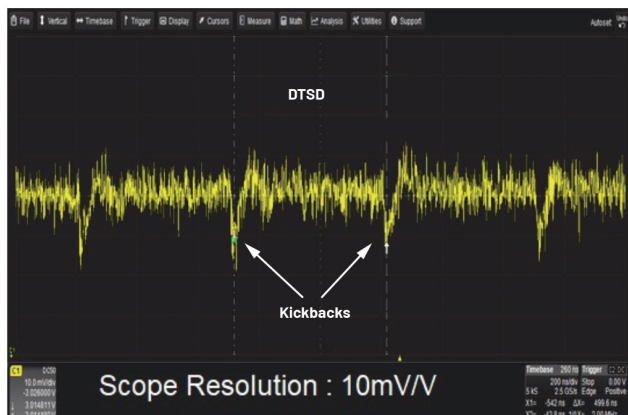
4. Kickbacks in input current for a DTSD ADC (a), and a continuous input current profile for a CTSD ADC (b).
