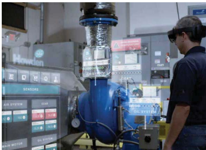
2. PTC's Vuforia can support viewing digital twins using augmented-reality glasses. (Courtesy of PTC)
