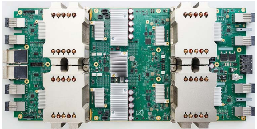
The second generation of Google's Tensor Processor Unit (TPU) for the data center.
