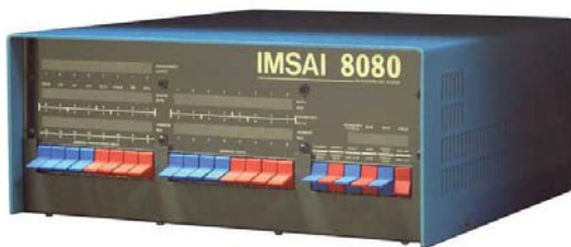
6. The IMSAI 8-bit Intel 8080 is built around the 8080 processor. (Courtesy of Intel)
