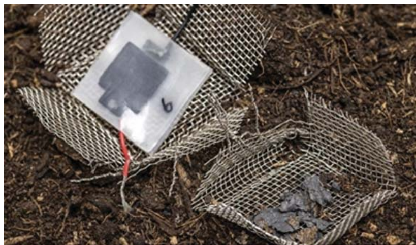
4. The capacitor disintegrated after two months buried in soil, leaving only a few visible carbon particles.
