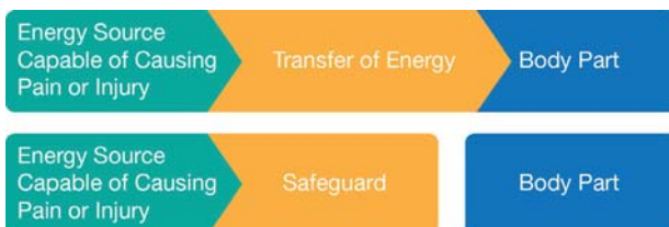
Figure 1: The HBSE three-block model shown is used to analyze energy classes, transfer mechanisms, and safeguards.
