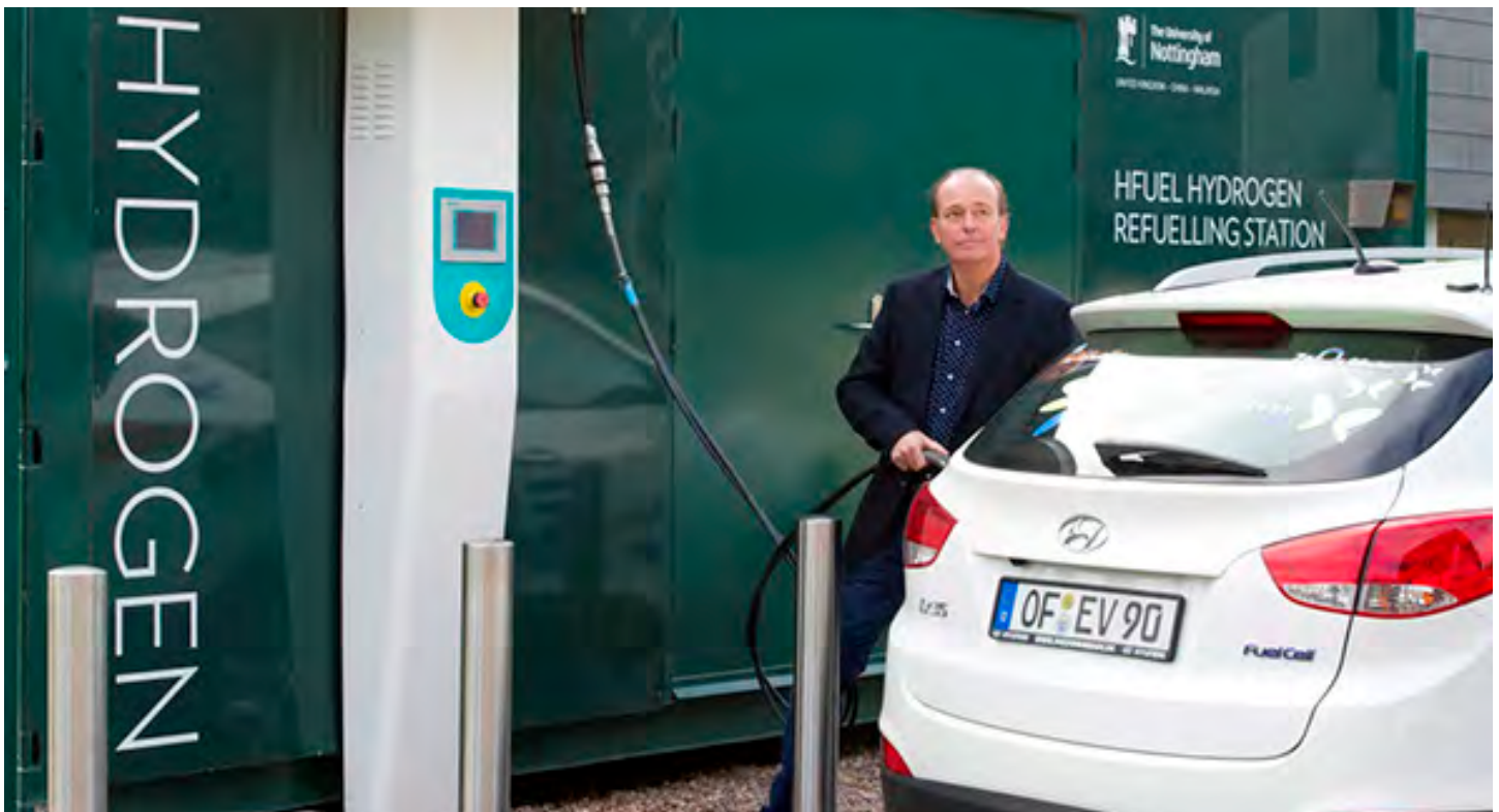
Re-fueling a Hyundai ix35 with hydrogen fuel. (Image courtesy of Bexi81 via Wikimedia Commons)
