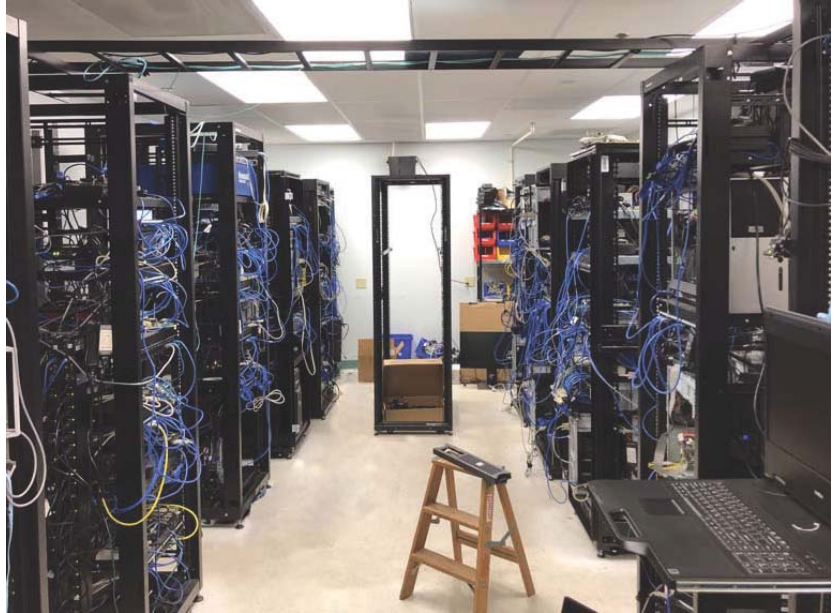
3. Green Hills Software's Embedded Board Farm allows remote developers to test real hardware.
