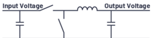
3. Concept of a simple buck step-down converter.
