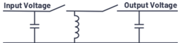
5. Concept of a simple inverting buck-boost converter.
