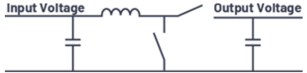
4. Concept of a simple boost step-up converter.
