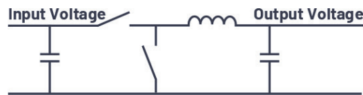
3. Concept of a simple buck step-down converter.
