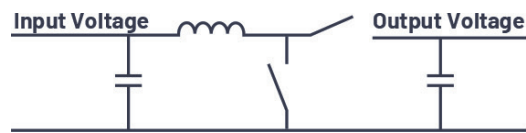
4. Concept of a simple boost step-up converter.
