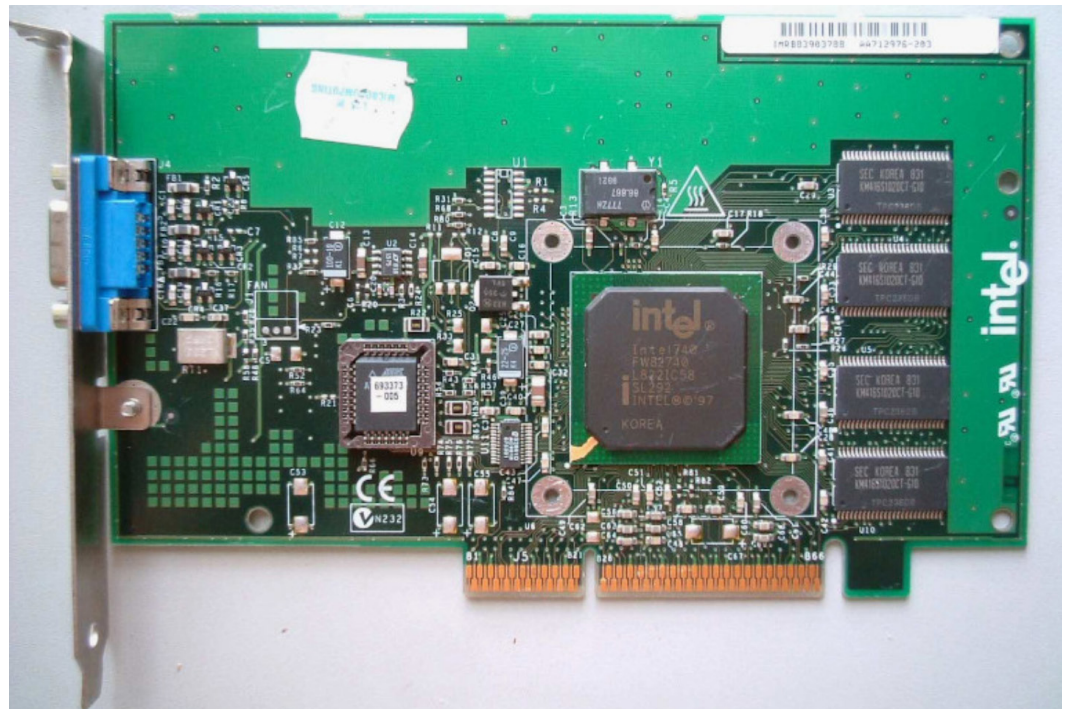
Figure 1. Intel i740 prototype AIB with AGP connector.
