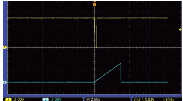
5. Trigger pulse and voltage ramp on capacitor C_X .
