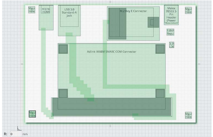
2. Developers can use Altium's Upverter online board designer to quickly create carrier boards.
