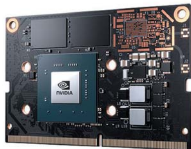
1. NVIDIA's Jetson Nano, with its 260-pin SO-DIMM connector, is plug-compatible with Xavier NX. Both can handle AI/ML chores.
