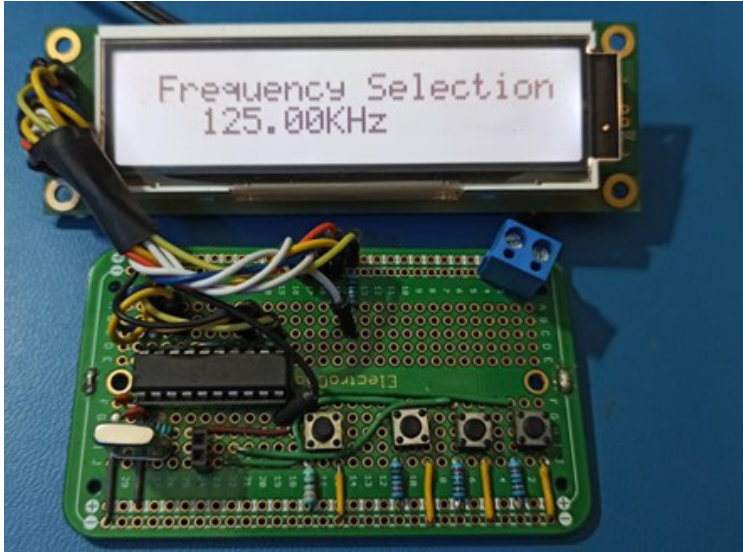
8. The LCD display shows a selected frequency of 125.00 kHz.
