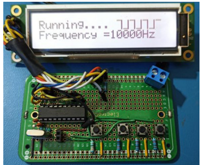
7. The LCD display shows 10,000 Hz is being generated by the microcontroller.
