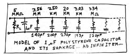
age is a big capacitor, in parallel with several small capacitors in series with various large resistors (see the figure). If we put a dc voltage on the capacitor for 0.1 second, some of those smaller capacitors will be charged up, but some of the bigger ones will take more time.
