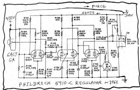
error of less than 150 µV ac rms. That's 100 dB of gain at around 120 Hz! Forty years ago, most regulator amplifiers had two-stage amplifiers. But this one used three dual triodes for each supply, + and - 300 V. Two honest stages of 12AX7 provide a lot of gain ( $\mu = 100$ ), and the  $12AU7 (\mu = 20)$  gives a good healthy drive to the grid of the output tube (6AS7GA).
