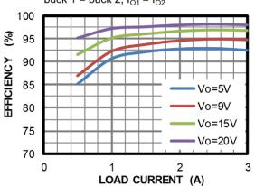
4. The MPQ4272 efficiency curve shows that an integrated solution can improve USB output voltage regulation as well as efficiency.
