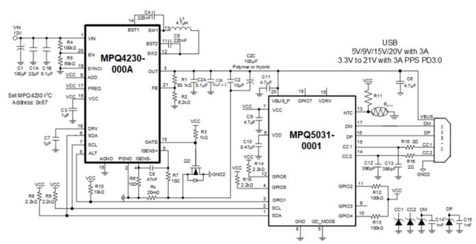
5. A 12-V V<sub>IN</sub>, 3.3- to 21-V V<sub>OUT</sub> solution for USB PD and PPS applications can regulate parameters while simultaneously allowing them to be adjusted.
