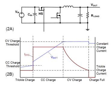
while the charge current gradually reduces). Figure 1 shows the charging profile of a Li-ion battery.
