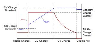
1. A lithium-ion charging profile has four charging phases: trickle charge, constant-current charge, constant-voltage charge, and charge full.
