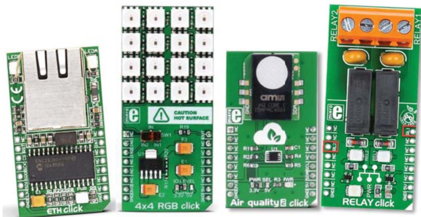
4. A range of Click boards are available from a number of sources; it's easy to design custom boards given the limited number of interface pins.
