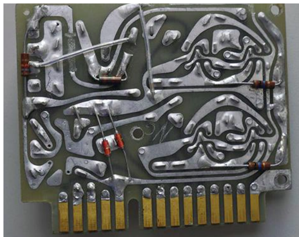
17. The backside of one of the prototype Philbrick cards, showing some cuts, jumps, and added components.
