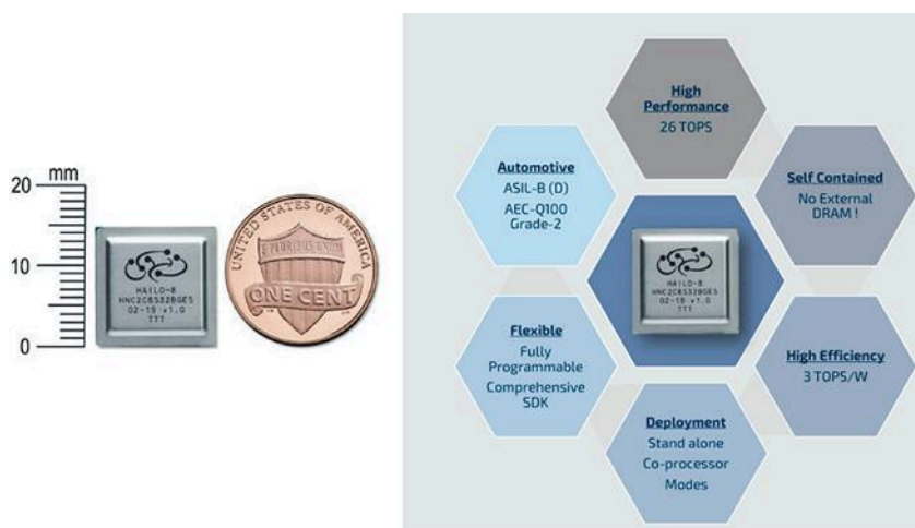
1. Hailo Technologies' Hailo-8 is a compact chip designed for rugged environments, including automotive applications.
