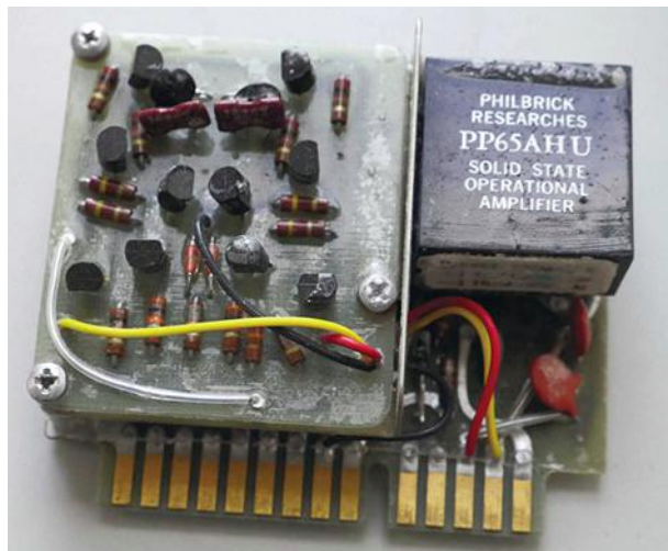
15. This mystery circuit card incorporates a Philbrick PP65AHU op amp.
