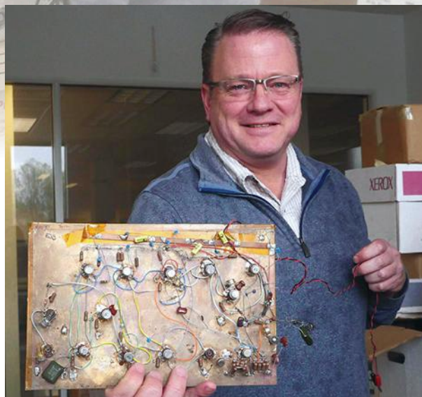
1. Texas Instruments application engineer Paul Grohe holds up an LM317 voltage regulator IC prototype likely designed by Bob Pease to improve the regulation accuracy over temperature.
