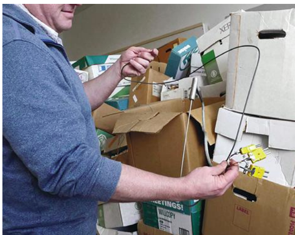
20. Paul Grohe shows the thermocouple assembly he helped Pease build.
