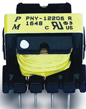
1. An example of a bobbin and core transformer for a 100-kHz switch-mode power supply.
