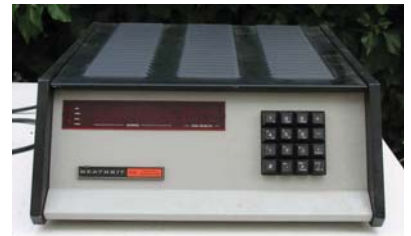
5. The Heathkit H-8 was an 8-bit microcomputer kit based on the Intel 8080A.
