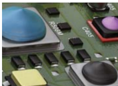
Whether automated or hand dispensed, Bergquist liquid materials have natural tack and precisely flow into position for a clean final assembly with little or no stress on components.
