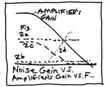
domain looking at Bode plots, the evaluation of loop stability is normally done in the time domain. Hit the input with a little step of current and see how well the output settles without excessive ringing.
