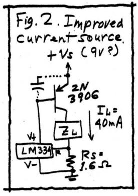
sistor will let you source 40 mA quite handily. And the voltage across the load does NOT have 0.7 V in series with it, so it regulates down MUCH better than Figure 1.
