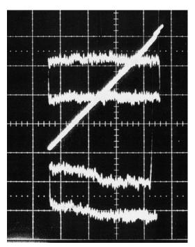
3. LMC6042, F = 0.6 Hz; output ±4 V into 1 k $\Omega$  (lower trace); upper trace, 2  $\mu$ V p-p at 20  $\mu$ V/div.; lower trace, 6  $\mu$ V p-p at 20  $\mu$ V/div.
