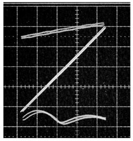
an LM301 can make a unitygain inverter with a nonlinearity of 1.2 ppm. At lighter loads, it's even better.
