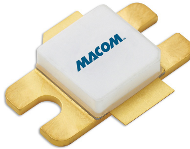
2. To make mmWave frequency semiconductors more affordable to consumers, GaN devices must be supplied in a variety of low-cost packages, including plastic packages. (Courtesy of MACOM)
