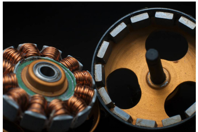
4. An outboard-type BLDC motor such as this one would produce trapezoidal back EMF.
