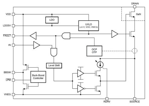
Texas Instruments' LMG341xR070 features a 600-V GaN transistor with 70-mΩ on-resistance. The internal gate driver has only 20-ns propagation delay and a 25- to 100-V/ns adjustable slew rate.
