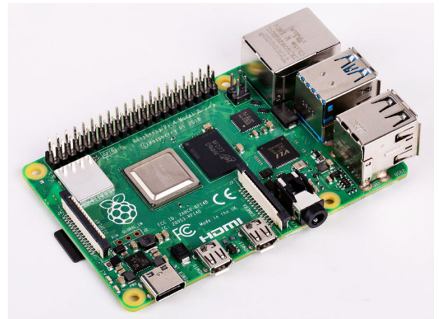
The Raspberry Pi 4 is the latest in a long line of compact application processor modules.
