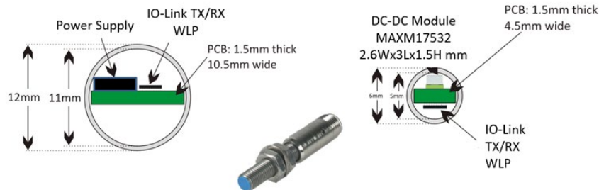
Tiny DC-DC converter power module provides most compact solution to fit in tiny sensor package
