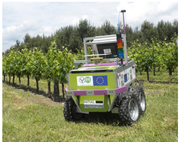
1. The AGV developed by the European VineRobot project uses non-invasive sensing technologies to monitor vineyards for vegetative growth, water status, and grape composition.
