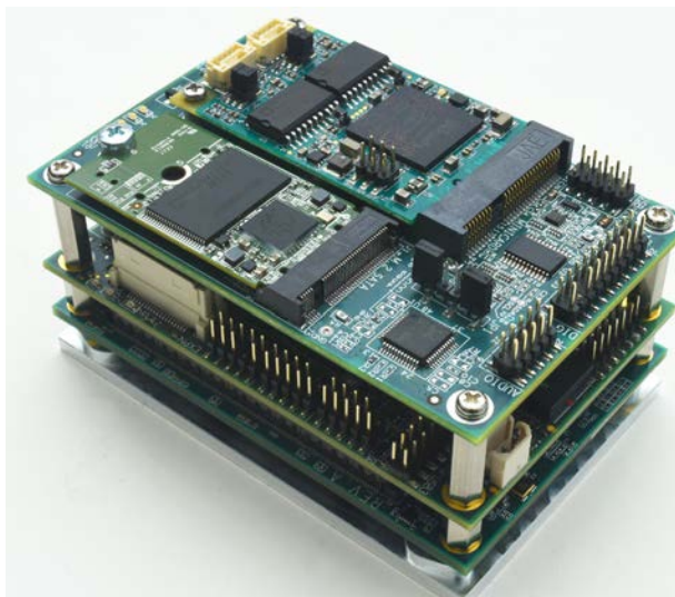
1. Diamond Systems Xeta COM Express SBC family can work with carrier boards that include Mini-PCIe and M.2.
