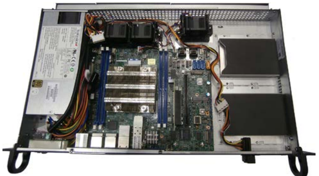
2. Supermicro 5019D-FN8TP system has a motherboard that includes an M.2 B Key socket and a Mini-PCIe socket with mSATA support.
