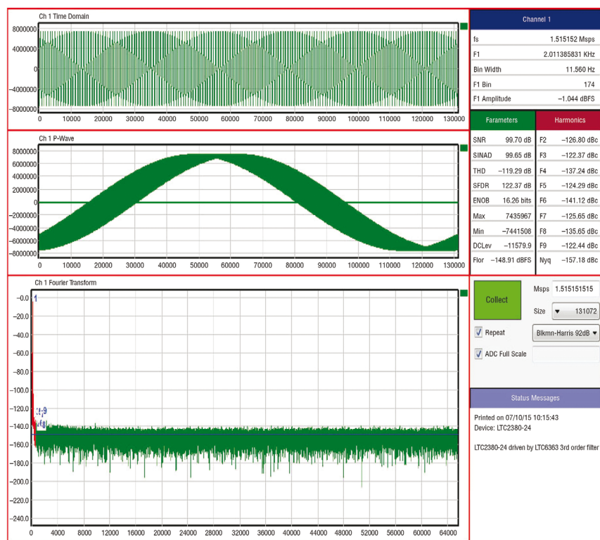
3. The PScope screen capture shows key parameters FFT, SNR, and THD of the circuit with N = 1 .
