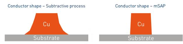
The rectangular shape enabled by the mSAP process is far more effective, maximizing circuit density and accurate impedance control with lower signal loss.
