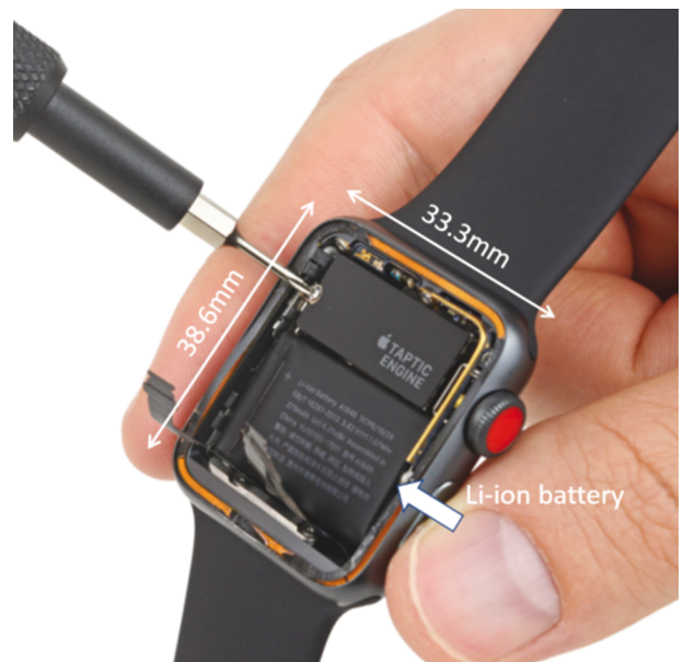
1. Like most wearables, the Apple Watch Series 3 leaves little room for its 279-mAh battery. Nonetheless, the watch can run for up to 18 hours with occasional use. Just be careful about talking on the phone—that can reduce the run-time to as little as one hour. (Source: ifixit.com)
