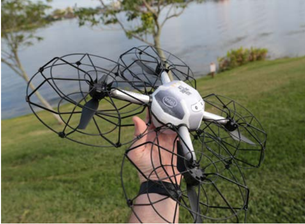
3. Intel's Shooting Star looks like a conventional quadcopter but it is designed to fly as part of a swarm.
