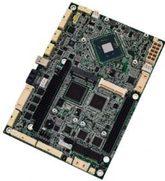
3. WinSystems' EPX-C414 motherboard has a pair of Mini-PCIe sockets and PC/104-Plus expansion.
