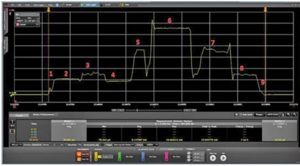
1. A plot of supply current vs. time during a wireless data transfer reveals distinct phases of operation.
