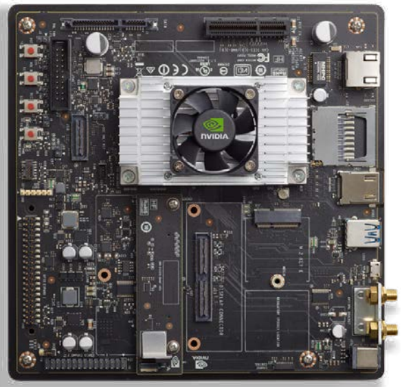
3. The Jetson TX2 development board is identical to its predecessor with the replacement of the module under the heat sink. Not shown are the wireless antenna connections between the module and the pair of antenna jacks in the lower right.
