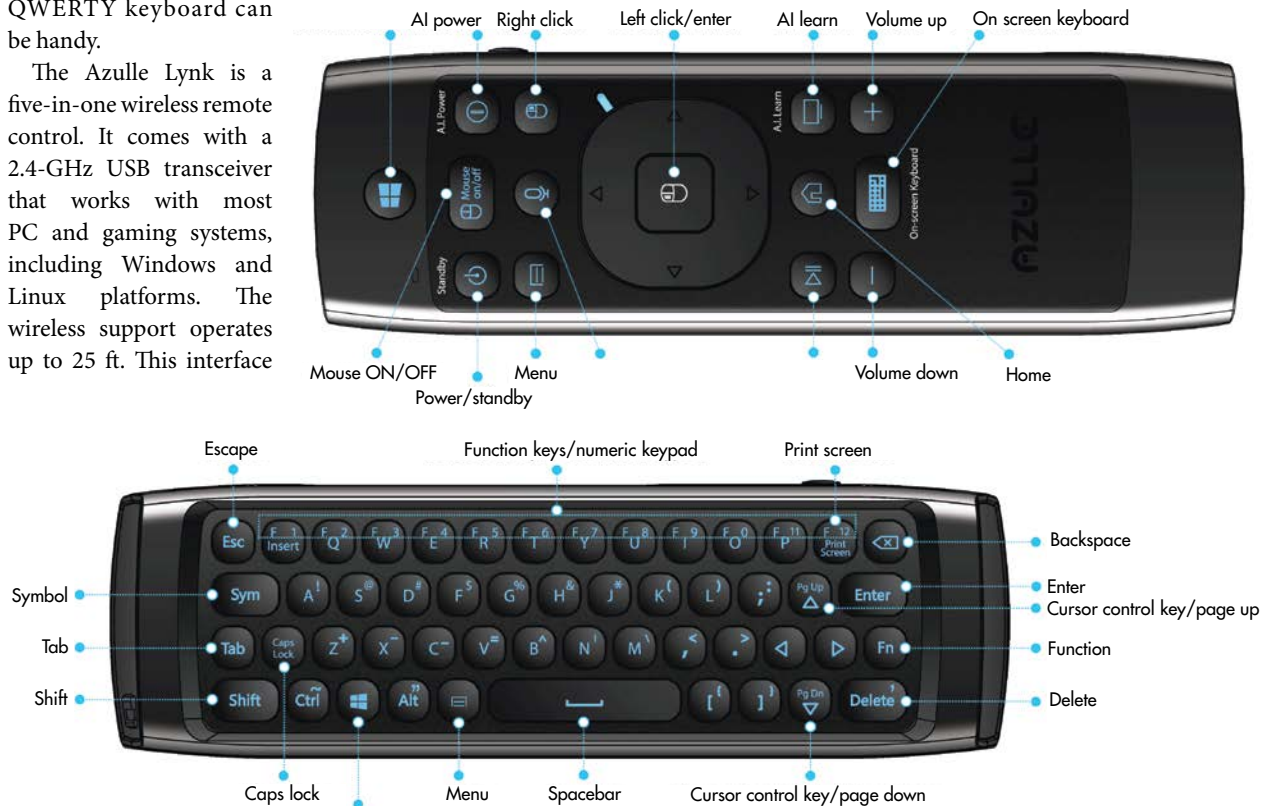
1. The Azulle Lynk is a five-in-one wireless remote control with a QWERTY keyboard on the back.
