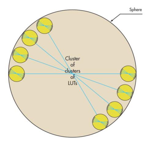
The higher layer interconnects the tiles with a matrix of tiny cross-bars, somewhat analogous to a network-on-chip (NoC) architecture, that sets this structure apart from the traditional mesh interconnection network. This approach ensures predictable, fast, and congestion-free routing.
