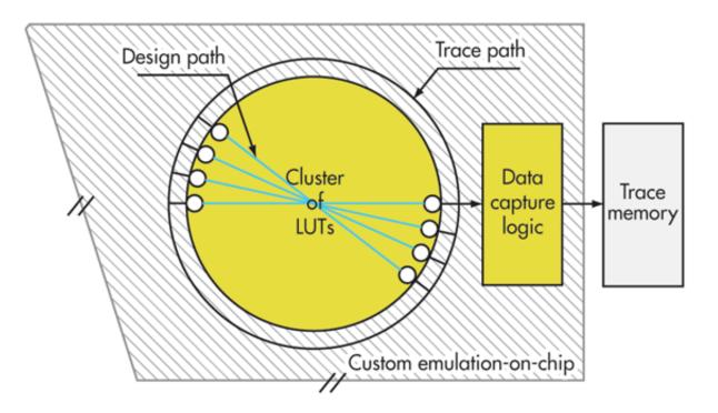
The design debugging capabilities are augmented by an integrated triggering mechanism and a built-in logic analyzer with a graphical path browser that accelerate the identification of difficult-to-find bugs. The emulator-on-chip enables triggering on registers by default, force-n-release, memory/register peek-and-poke, and save-n-restore.
