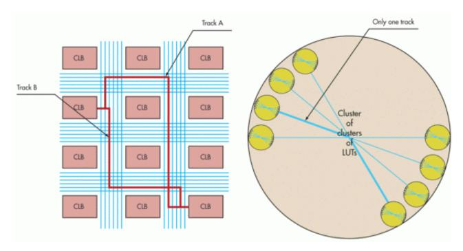
The multi-layer interconnection network trades off high capacity, now available in the largest FPGAs, in favor of fast and congestion-free FPGA placing and routing (P&R). It is possible to place and route one custom FPGA in about five minutes. Even by lowering the filling rate of the largest FPGAs to 50% or below, the P&R may take a few hours.
