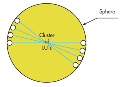
Extending the analogy one hierarchical level higher, clusters of LUTs may be distributed on the surface of a larger sphere and interconnected with the same scheme (*Fig. 3*). Basically, it's a fractal graph where the same pattern is repeated, moving from the outside to the inside or from the inside to the outside. The higher layer interconnects tiles with a patented structure that offers similar benefits inherent to the lower layer.
