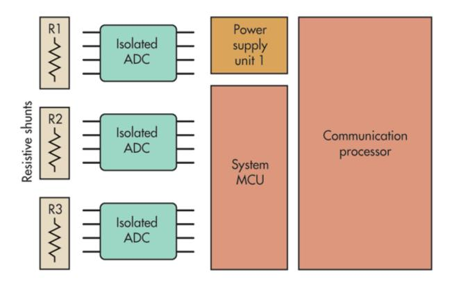
When semiconductor suppliers leverage chip-scale transformer technology and advanced converter technology within the same IC package, smart meter systems achieve a new level of integration, performance, and reduced overall cost. It is relatively easy to tamper with a CT by placing an external permanent magnet close by, ultimately causing the smart meter to undercount or stop working altogether.
