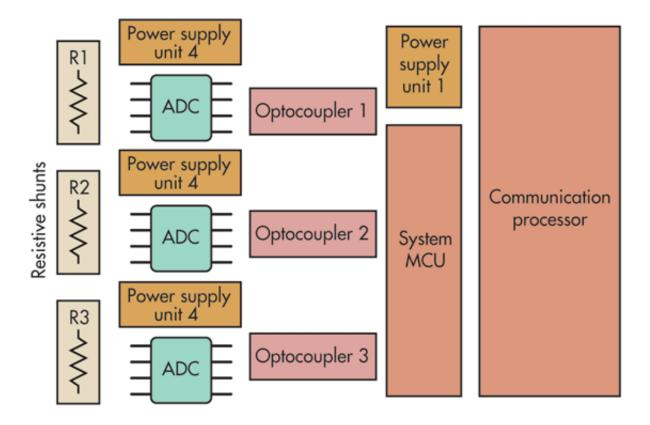
Chip-scale transformer technology now makes it possible to isolate not only data channels but also the power domain so the system can be completely separate. With its very small size and very high manufacturing reliability, it can be combined with other smart meter blocks all within the same IC package. The result is a new polyphase smart meter architecture (*Fig. 5*).
