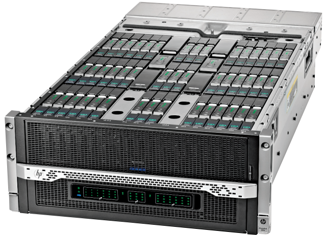
4. HP's Moonshot provides a number of high-speed fabric interconnect options between processor boards.
