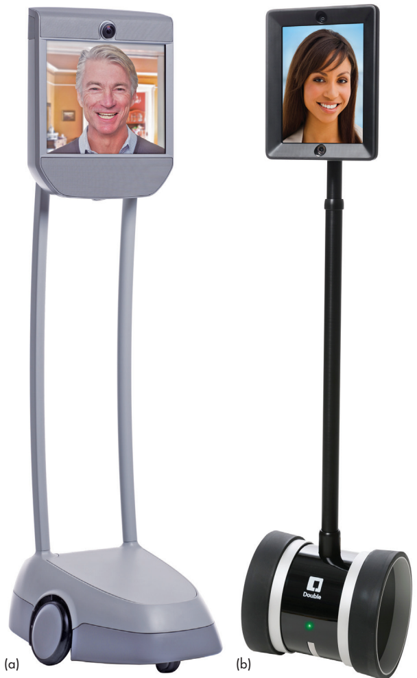
1. The Suitable Robotics Beam (a) and Double Robotics Double (b) are just a couple of telepresence devices that are becoming more common in everyday life.
