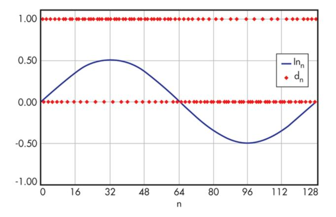
For the example, the stream still remains with single lows for positive input and single highs for negative inputs. The average of the 128 outputs is zero, and there are 44 rising edges for an  $f_{Out}$  of 44/128 or 34.4%. The equivalent input to generate 44 inputs would be an input dc of 1/PI(). Since the average of this sinusoid rectified is, in fact, 1/p, the output frequency can be used to measure the average of an rectified signal.
