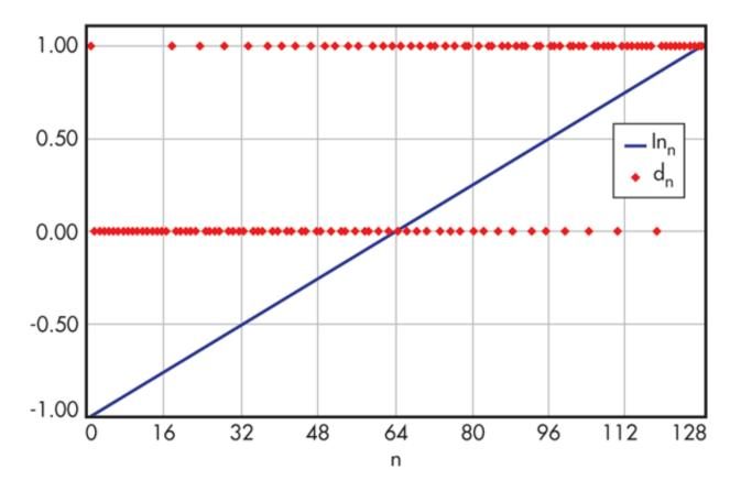
The spreadsheet provides a lot of interesting data. When the input is negative, the output stream is more lows followed by a single high. For positive inputs, the opposite is true. There are 32 of rising edges, which is the same value obtained when the input was +0.5. The average of the absolute value of this signal is 0.5.
