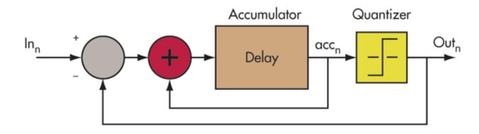
The accumulator is built from a clocked register that feeds back to itself. Here it is called delay, but it sometimes is called a register or  $z^{-1}$ . I like the term "previous." For this block diagram, acc is equal to the previous acc plus the previous in minus the previous out. Also, out is a function in the acc. Stated mathematically:
