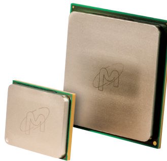
12. The HMC package is designed to deliver a 15x performance improvement over existing DDR3 modules while using 70% less energy.
