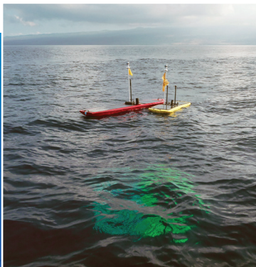
1. The Wave Glider consists of a floating section near the surface and an energy harvesting and traction system that is connected by an umbilical cord.
