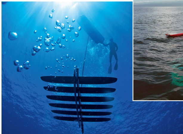
1. The Wave Glider consists of a floating section near the surface and an energy harvesting and traction system that is connected by an umbilical cord.
