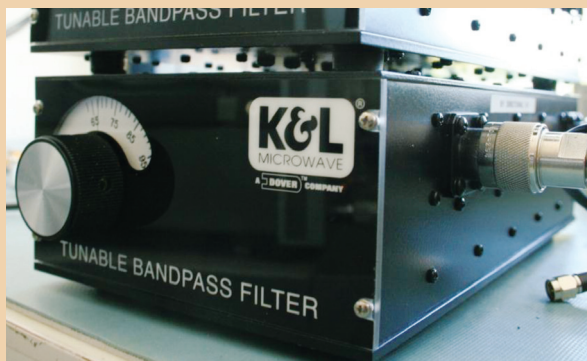
2. Before the test signal reaches the circuit in Figure 1, it goes through a tunable bandpass filter. The lower filter is used for the signal path, and the upper handles the clock signal.
